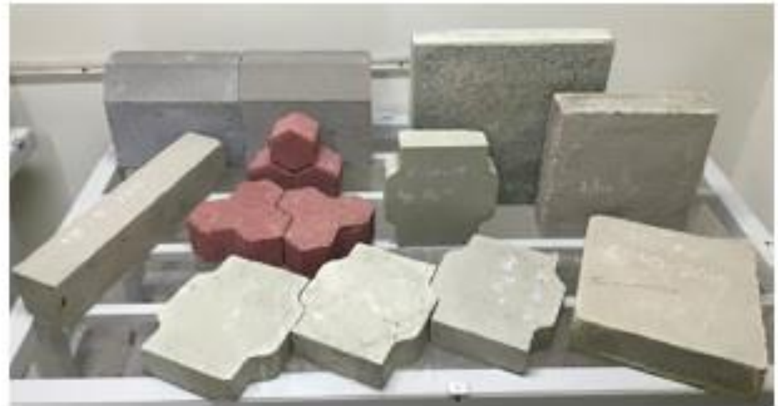
Fig. 6. Sulfur concrete products in contrast with conventional concrete and sand cement products.
