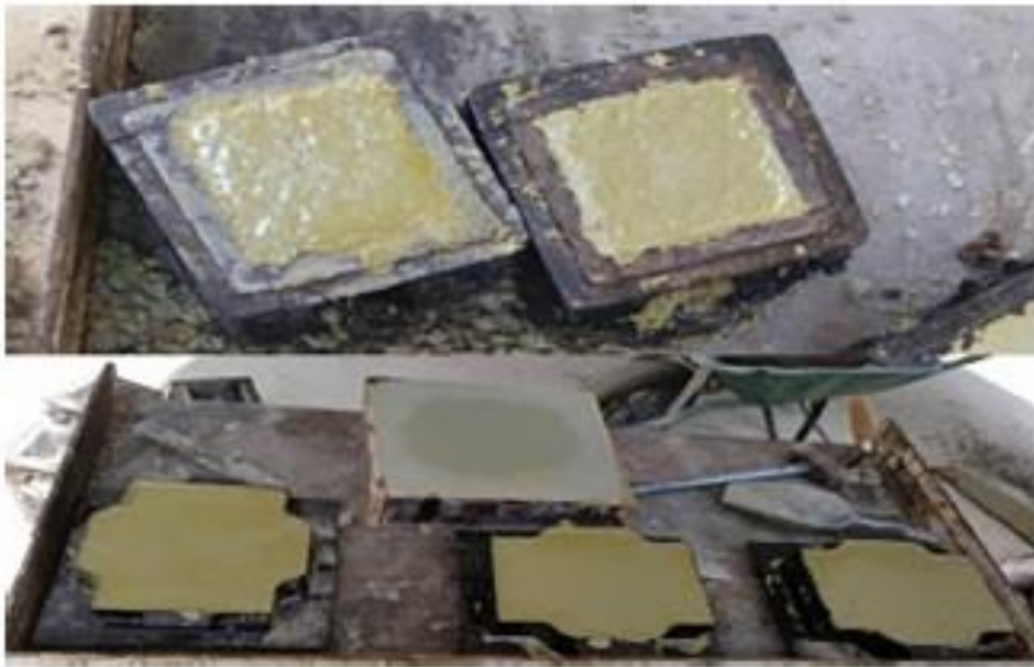
Fig. 5. Cast solidified sulfur concrete specimens set for curing.
